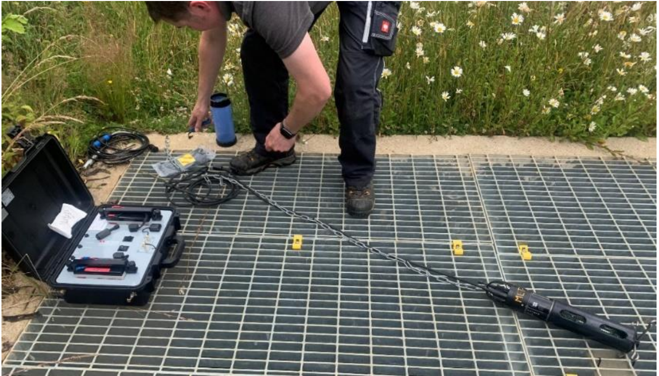
Figure 2.6: Image of the inlet sonde being installed for the summer monitoring period.
